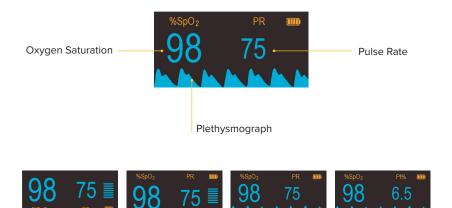
SpO2, Pulse Rate and Pulse Rate Bar, Plethysmograph Waveform, Perfusion Index and **Battery Status Indicator**
